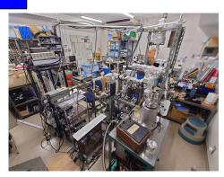
To determine the age of a sample using the K-Ar dating method, we employ two instruments in our laboratory. The first one is a flame photometer (left), which measures the sample's potassium amount. The second instrument is a noble gas mass spectrometer (right), which is used to measure the ratio of argon isotopes. We also have equipment for mineral separation, such as an isodynamic magnetic separator and sodium polytungstate (SPT) heavy liquid.
